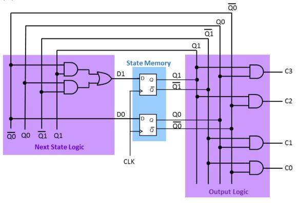
(iv) Comparing this implementation to T8Q2, it can be seen that while less FFs are required, more logic gates are used (complexity has increased). However, less FFs imply a smaller area or cost. Assuming the same timing characteristics for the D-FFs, the maximum operating speed of this counter would be slower due to the need to cater for additional logic gate delays from the next state logic block.
